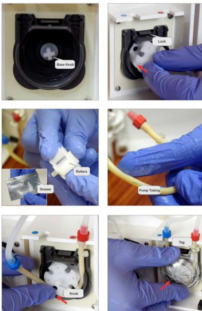
Figure 3: Pump tube installation procedure
